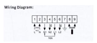
Connect the floor sensor, power leads and load leads.
